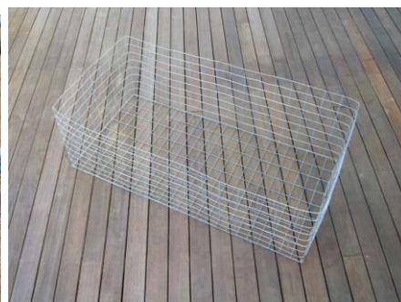
The frame complete but without the stabilising wire.
